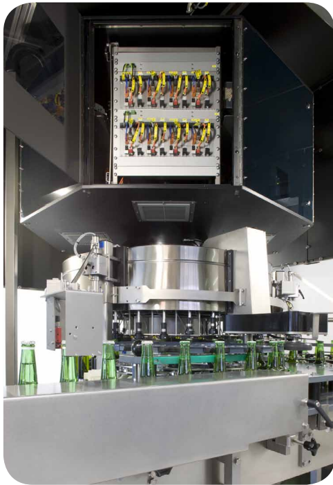
Figure 2: The 'blank slate' principle provides exceptional application flexibility and easy integration. This picture shows a high end system with a total of 8 camera systems on two levels.
