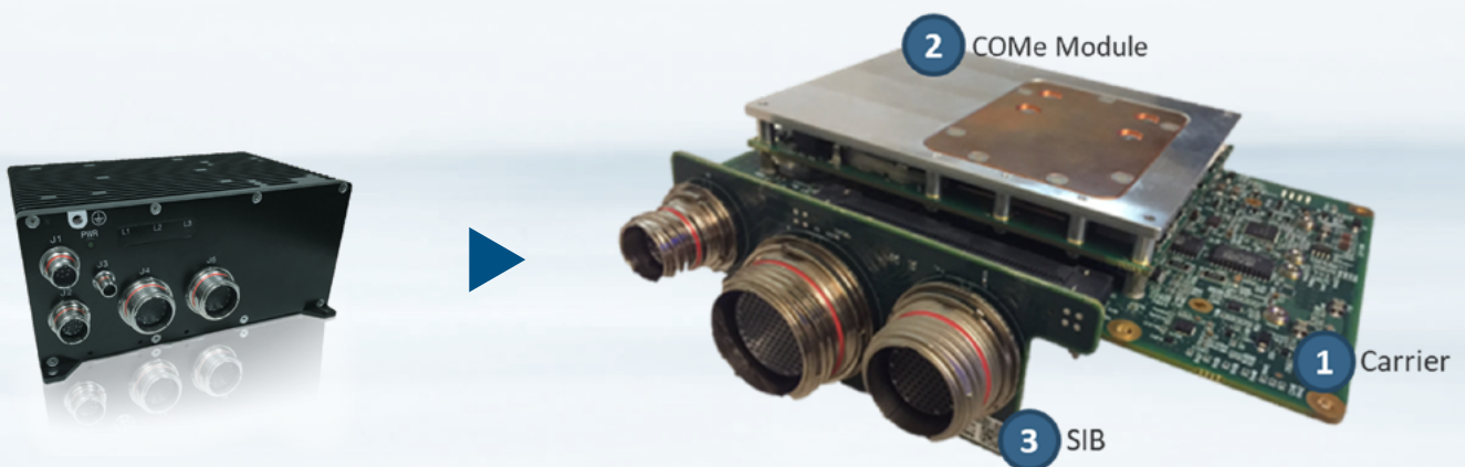
// Components of a typical Integrated Mission Computer. The carrier card (1) hosts the COM Express®-based computing module and heat spreader, along with the front-panel Signal Interface Board (or, SIB). This arrangement permits a range of onboard and front-panel customization options.
