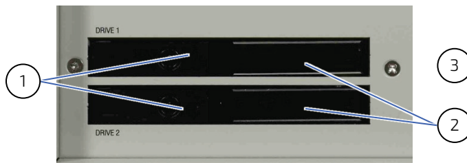
Figure 18: Drive 1 and Drive 2 for removable 2.5" SATA HDD/SSD (option); closed drive bays
