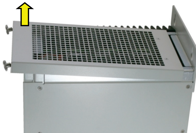
Figure 37: Removing the cover (detail of the KBox C-104-TGL-2)
