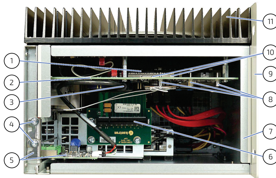
Figure 41: KBox C-104-TGL-2 - internal view with COMExpress® module and with PCIe riser card
