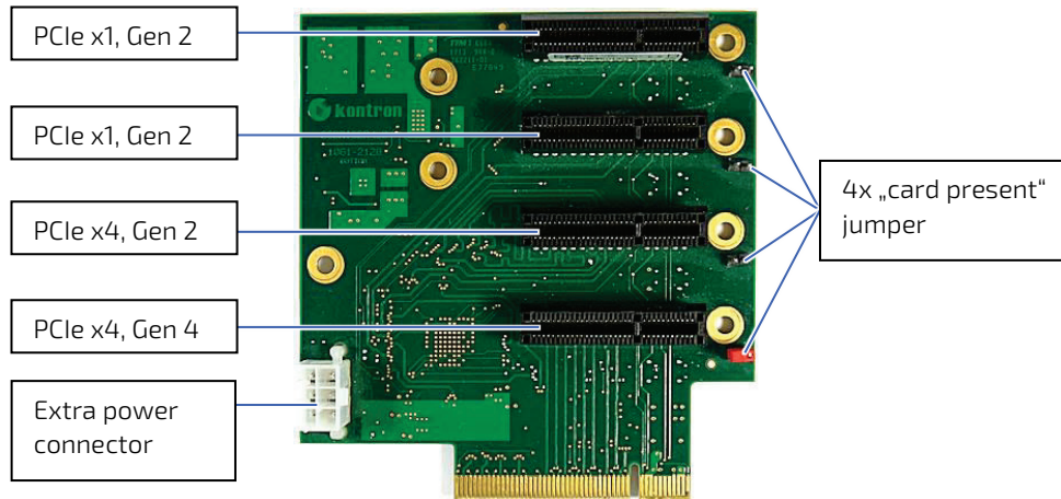
Figure 42: Riser card with 2xPCIe x4 and 2x PCIe x1 slots for KBox C-104-4
