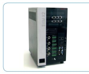
Image 3: Kontron ships the Box PC for the Seidenader SV360 solution tailored to meet Seidenader's individual requirements. It comes with six Firewire connections (currently a maximum of three asynchronous Firewire cameras is planned on the I/O board), various I/Os (trigger, strobe, GPIO) and two storage media in a RAID array.
